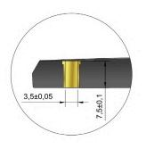
To achieve the optimal performance locate the tag on metal in a way that there is metal on both ends of the tag. Ideally the tag is placed on large even metal surface with direct metal contact underneath the whole tag. Tag polarization is along the longest dimension. This should be taken into account when using linear polarized reader antennas.
