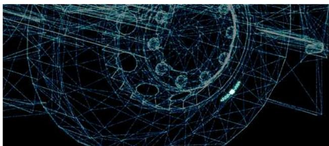
Embedded RFID TireTag offers more flexibility with small size and omni-directional antenna design
